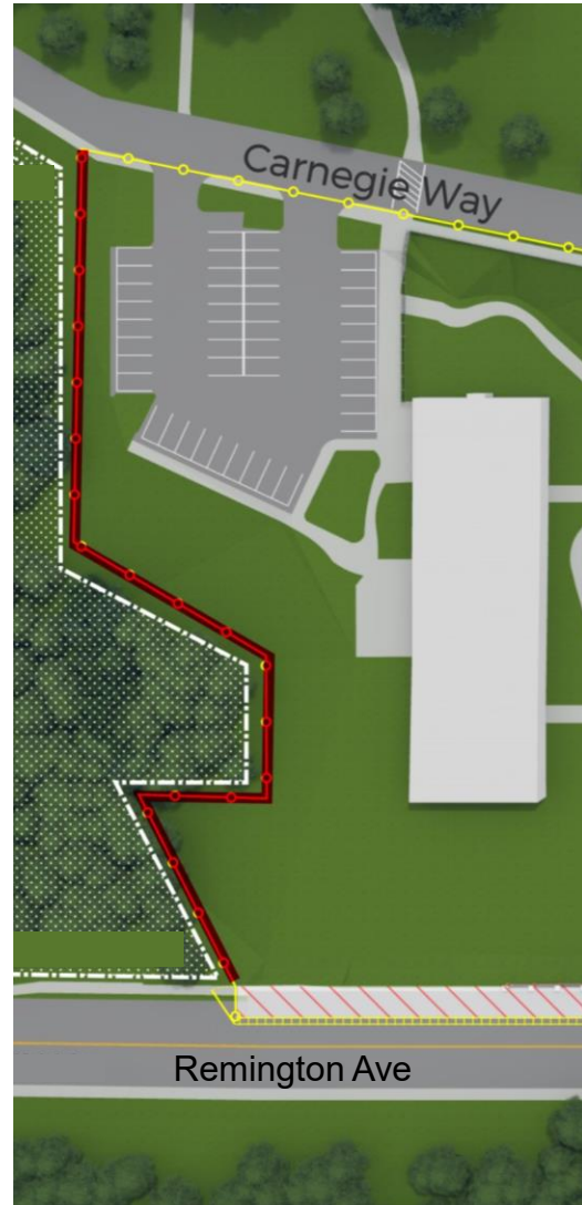
Red Line: Construction Fence and Super Silt Fence
