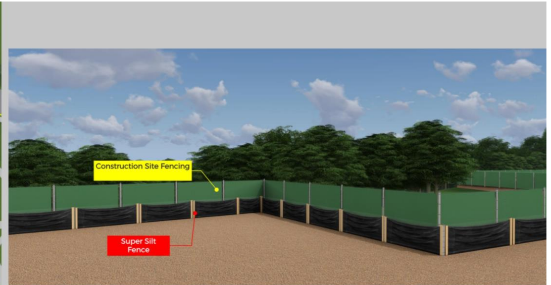
Super Silt Fence Details
